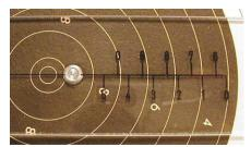
for ease of reading. The gauge is inserted in the target in the same way as the decimal gauge. However in this case the number of tenths to be added is determined by which of the numbered, engraved lines aligns with a line on the target. If no line aligns accurately, then the value is that of the nearest line *just inside* a scoring ring on the target, e.g. 10.1 in the illustration above.
