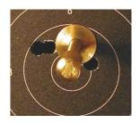
adjacent to the shot-hole. This may be because the scoring ring has been struck or otherwise damaged by the bullet, other adjacent shot-holes or splashback. In these cases, it is possible to use a gauge with an over-sized flange to determine the shot value by reference to another ring on the target.
